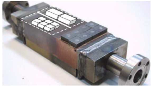
Fig. 9. Actively-cooled Be armored mock-up with cast CuCrZr layer (successfully withstood 2000 thermal cycles at 7 \text{ MW m}^{-2} ) (RFPT).
